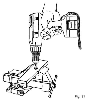
When drilling hard smooth surfaces use a center punch to mark desired hole location. This will prevent the drill bit from slipping off center as the hole is started. However, the low speed feature allows starting holes without center punching if desired. To accomplish this, simply operate your drill at a low speed until the hole is started.
